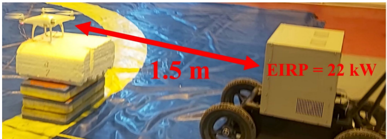
Fig. 9. High-Power Wave Radiation Device Operating at 2.45 GHz with EIRP = 22 kW CW for Phantom Exposure.
